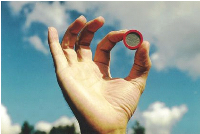
Figure 1 Passive sampler as distributed by IVL
